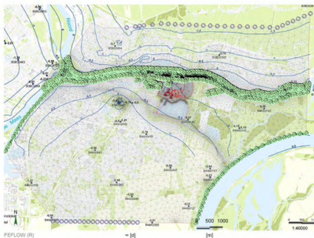
Figure 3-6: Existing Moria Model and definition of the BC (see Figure 3-7 for BC legends)
