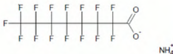
Figuur 4.7 Evenwicht na oplossing APFO in water (PFOA anion en ammonium kation) (Bron: ECHA 37 )
